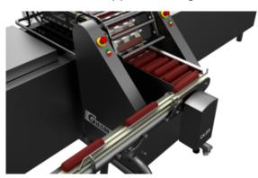
with clips. With a stickbuffer the sausages (with clips) can be loaded directly into the buffer or a connecting belt can be used when space next to packaging machine is not sufficient. For de-clipped products the connecting belt is used to place declipper in front of packaging machine.
